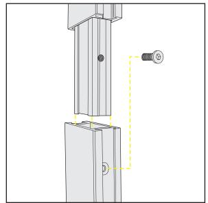
Inline Connection between Extrusions
