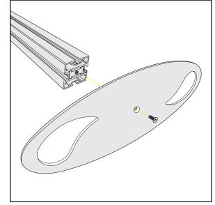
Baseplate Connection for Vertical Extrusions
